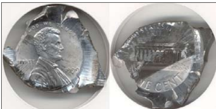
1999 Lincoln Cent Struck on Feeder Finger Tip ANACS MS 65
