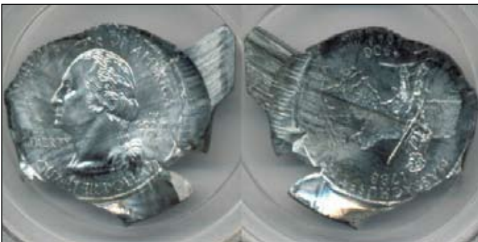
2000-P Massachusetts Quarter Struck on Feeder Finger Tip PCGS MS 65
