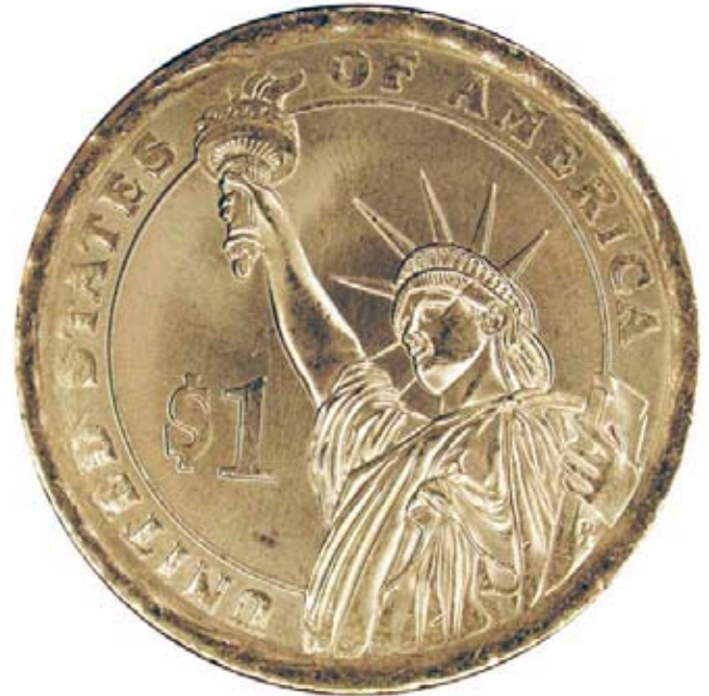
Photos #6b. The reverse of this Monroe $1, missing obverse clad layer, shows characteristic weakness around its rims.
