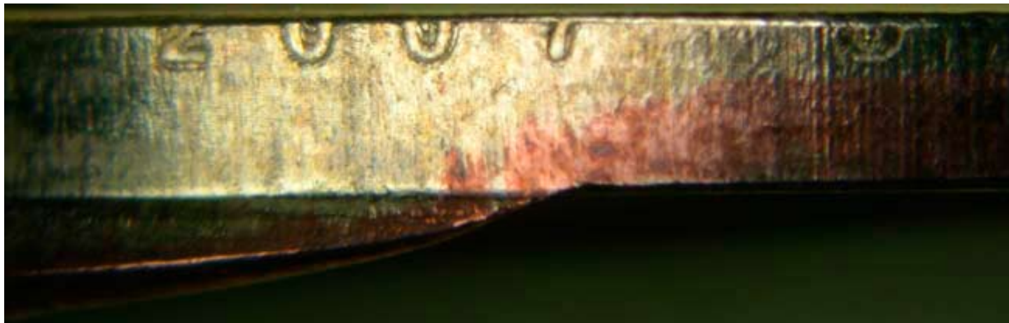
PHOTO #3b: View of edge of proof 2007-S James Madison $1 partial collar error, showing high position of the date, 2007. The raised flange can also be seen at the left hand side of the image.
