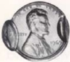
1965 LINCOLN FLIP-OVER AND DOUBLE STRUCK AT 9:00. INDENTED STRIKE, PARTIAL COLLAR. VERY UNUSUAL. CHOICE BU $45.00
