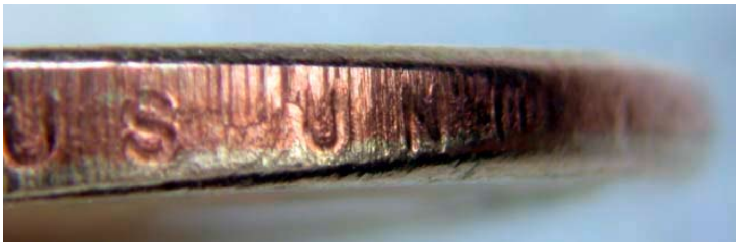
PHOTO #1d: View of edge of proof 2007-S John Adams $1 struck from horizontally misaligned dies, showing wedge-like shape.
