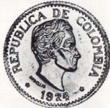
1924 COLOMBIA 5 PESO GOLD. NEW TYPE OF ERROR. HUB DROPPED ON WORKING DIE AND IN TWO AREAS; ON NOSE AND IN FIELD. BU $70.00
