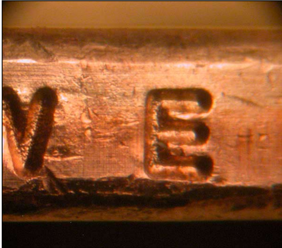
Photo 1: This is a genuine lettered edge Washington dollar with the smooth edge and fine vertical lines created when the coin was ejected from the collar after being struck.
