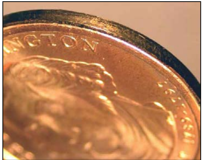
2b.) Close-up of the edge of a George Washington Presidential $1 coin missing edge lettering
