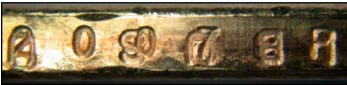
Photo #2b: Close up of edge, showing the inverted doubled edge lettering.
