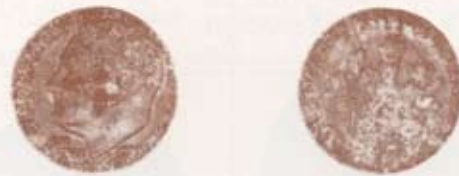
197X ROOSEVELT DIME. COPPER CORE ONLY! BOTH LAYERS OF COPPER-NICKEL SPLIT-OFF BEFORE STRIKING. WEIGHT IS ONLY 16.3 GRAINS.
