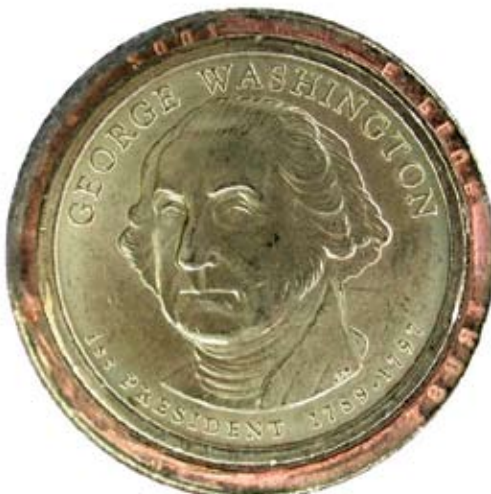
Photo #3d: Partial Edge lettering. Several portions of the edge legends are missing, and mint caused damage is evident.
