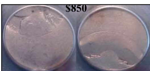
1941 5c Multiple error: Die adjustment strike struck 50% off center. PCGS AU 50
