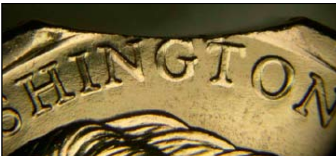
Photo #12b: 5% curved clip, a close up of the clipped arc. Note how the metal on the letters 'NGT' flows toward the clipped area.
