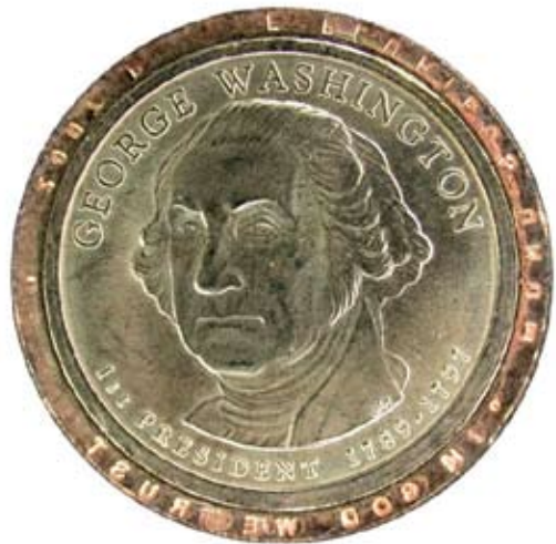
Photo #2b: Improperly spaced edge lettering. Note the irregular gaps between legends.
