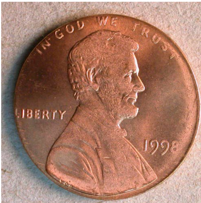
Figure 2. A 1998 cent struck on a copper-plated zinc planchet intended for another country. It weighs 1.73 grams.
