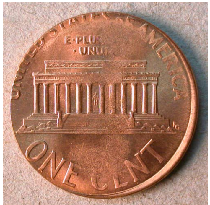
Figure 2. A 1998 cent struck on a copper-plated zinc planchet intended for another country. It weighs 1.73 grams.
