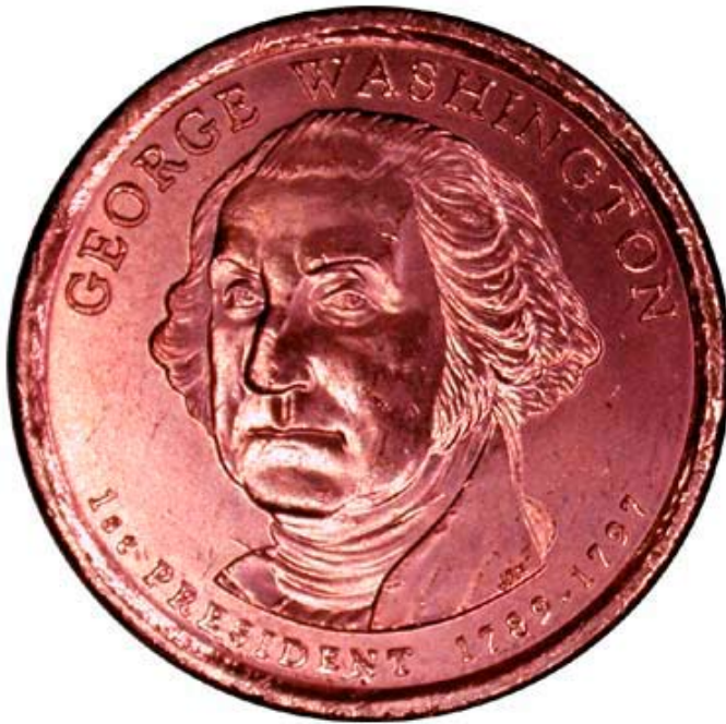
Photo #5a: Obverse missing clad layer.
