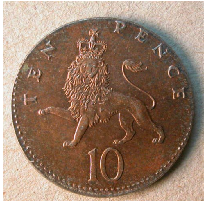
Figure 4. A 1992 British 10 pence struck on a steel planchet with a light and incomplete coating of copper.
