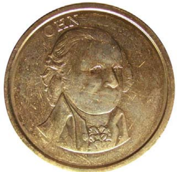
Photo #4: John Adams $1, obverse struck through. The dies are filled with grease, dirt, or metal particles causing a significant loss of design.
