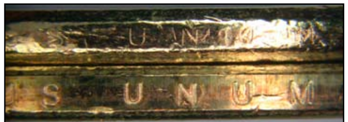
Photo #11b: Weakly lettered edge planchet, top, compared with regular edge lettering on bottom.
