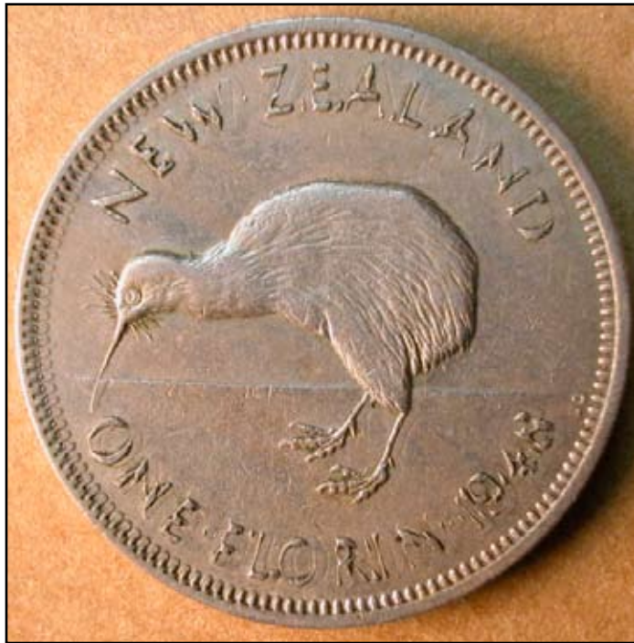
Figure 2a - Reverse face of a double-struck 1948 New Zealand 1 florin coin with a rotation of the hammer die on the second strike.
