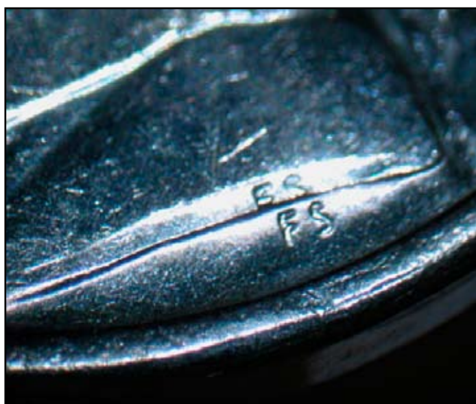
Figure 3c - Close-up of the base of Jefferson's bust showing duplication of the designer's initials.
