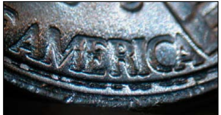
Figure 6c - Close-up of the affected area, showing an extra set of letter tips from AMERICA.
