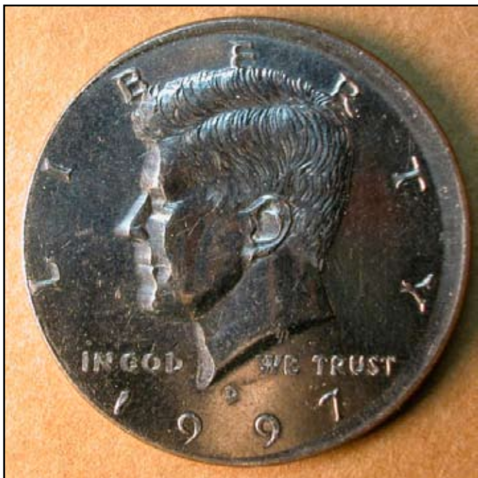
Figure 4 - A 1997-D half dollar with severe machine doubling (“slide doubling” subtype) on the obverse face.
