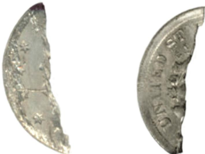
The blanking press takes the coils of metal strips and punches blanks out of it, ejecting the webbing at the other end. The webbing is cut into small scrap pieces to be melted and recycled. Occasionally a scrap piece will be mixed with the blank planchets and struck by the dies. Struck fragments are rare in the larger denominations. These can be uniface or die struck both sides and are very rare on type coins.
