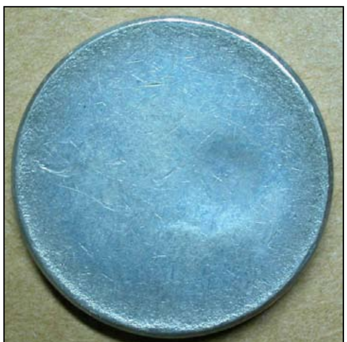
The obverse shows a shallow, circular strike-through error. It lies opposite the island of die-struck design on the reverse.
