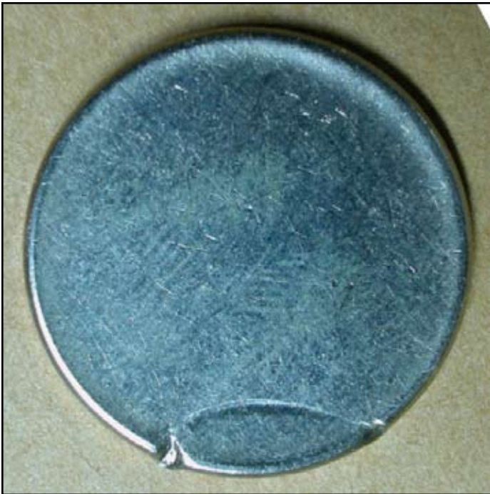
Shallow groove on the obverse of a 2005 West Virginia quarter with an “invisible strike”. This strike-through error is probably from a machine part or piece of hardware. Coin discovered by Gregory Capps.
