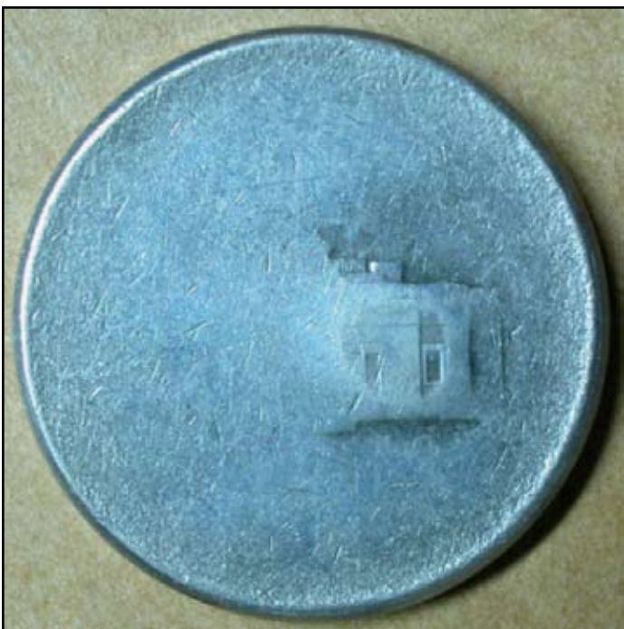
Reverse of an invisible strike nickel showing an isolated region of Monticello. Coin acquired from Rich Schemmer.
