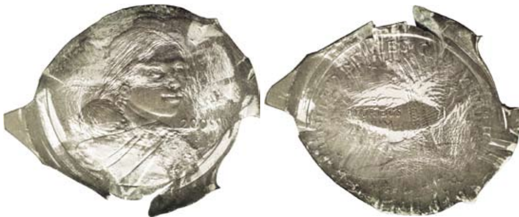
2000-P Sacagawea Dollar--Multiple Strike on End of Feeder Finger--MS65 NGC
