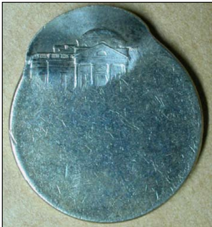
Reverse of an invisible strike nickel that was struck 30% off-center but which shows only the outer portion of the strike. Coin acquired from Paul Burrell.
