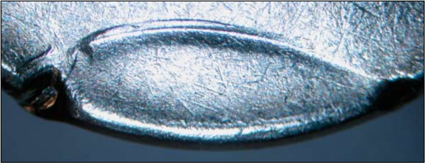
Close-up of the groove and the two angular indentations at each end.
