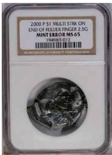
2000-P Sacagawea Dollar--Multiple Strike on End of Feeder Finger--MS65 NGC
